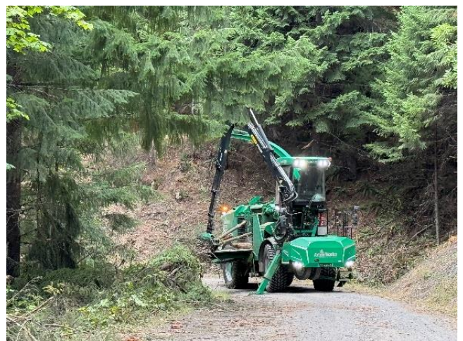
A self-loading chipper works to remove fuel along a roadway. Photo credit: Steven Kraus
