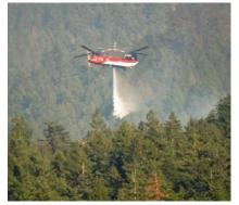
Chinook "heavy" helicopter drops water in the Coal Creek drainage on October 16, 2022. This helicopter uses a snorkel system to pull water from a lake or river to fill an internal tank. Other helicopters on the fire use a bucket system to scoop water.
