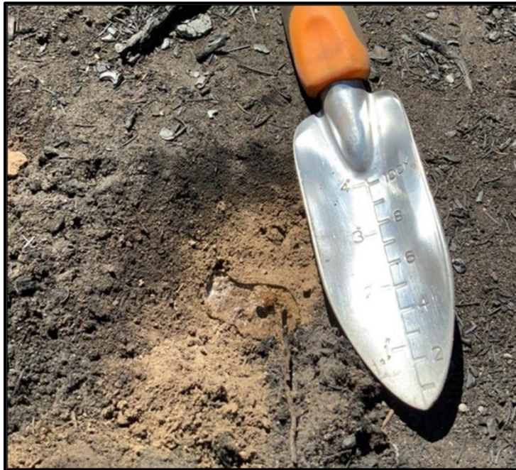
Figure 5: Strong hydrophobic soil conditions caused by moderate soil burn severity in mixed conifer forest. Note 2 cm diameter water drop that persists on soil surface.
