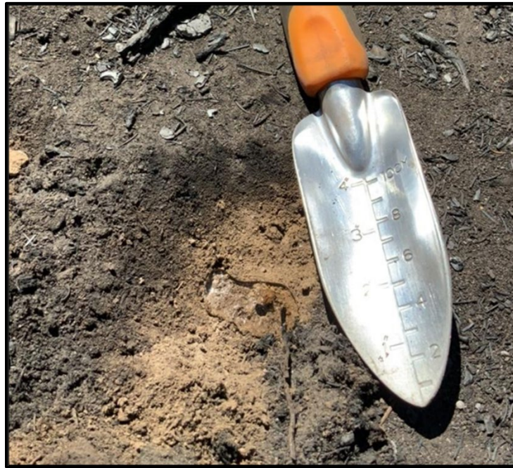
Figure 4: Strong hydrophobic soil conditions caused by moderate soil burn severity in mixed conifer forest. Note 2 cm diameter water drop that persists on soil surface.
