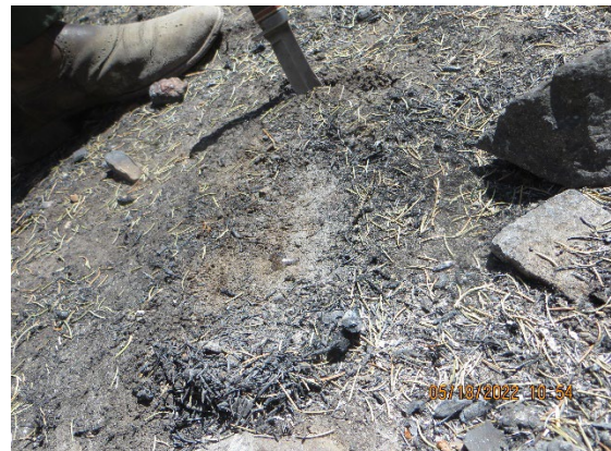
Photos 7, 8, 9 : BAER team soil scientist Mike Natharius testing for soil hydrophobicity. Mike captures a drop of water placed on the burned soil which was determined to be hydrophobic.
