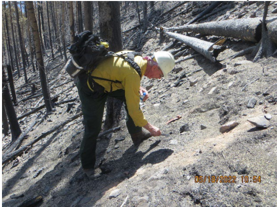
Photos 7, 8, 9 : BAER team soil scientist Mike Natharius testing for soil hydrophobicity. Mike captures a drop of water placed on the burned soil which was determined to be hydrophobic.
